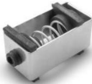
Range designed for suspensions of suspended acoustic ceilings and machinery working at more than 450 r.p.m. Manufactured with piano tail quality spring of great mechanical resistance guided by two rubber plates with integral end stops to prevent contact between spirals when overloading.
